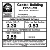
†For more information, please see *Your Guide to Common Household Condensation* at gentek.ca. ††Simulations performed by Enermodal Engineering Ltd. using Window 5.2 and Therm 5.2 as per NFRC100-2001. Outside temperature 0°F, inside temperature 70°F. Low-E glass Cardinal Low-E² 272. Air spaces .500° wide, 90% argon fill. IGU's 24" x 48". The secondary butyl used with Intercept was 0.035' thick. The conductivity used for Super Spacer Premium was 0.102.
